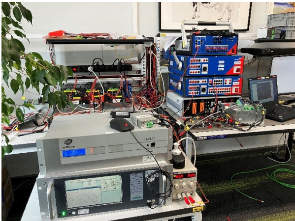
Fig. 5. Measurement setup for testing the SAMU
